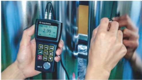
壁厚测量 Wall thickness measurement
