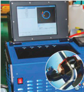
管道TIG自动焊 Pipe TIG automatic welding
